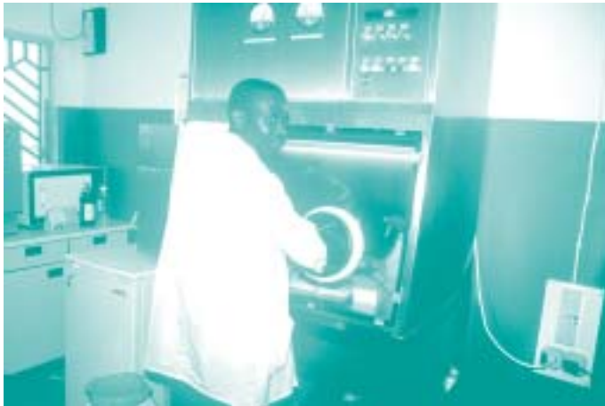
BSL3 glove box: Inside the PFHG-laboratory: Biosafety level 3 glove box for handling of highly infectious material
